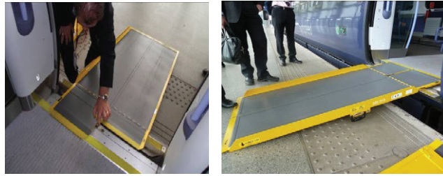
Fig. 1. Vehicle-based ramp as used on UK South Eastern Trains, King's Cross St. Pancras Station, London
