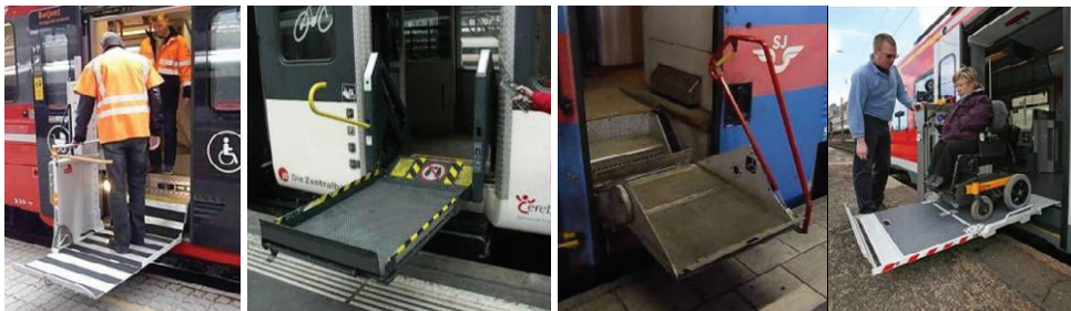
Fig. 2. (a) Example for vehicle based lift in Norway; (b) in Switzerland; (c) in Sweden; (d) in Germany
