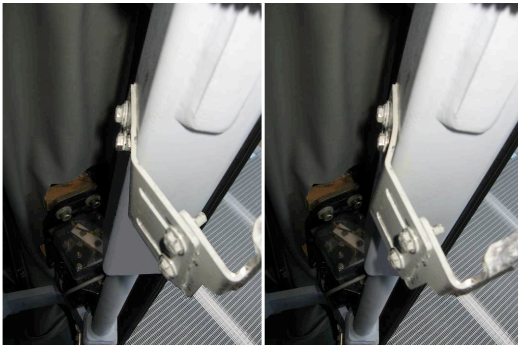
fig. 21 retention brackets (a) not deformed; b) deformed)
