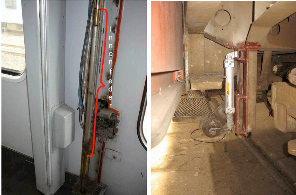
fig. 7 The mechanical power-shaft (left) replaced by a pneumatic drive underneath the vehicle floor (right)
