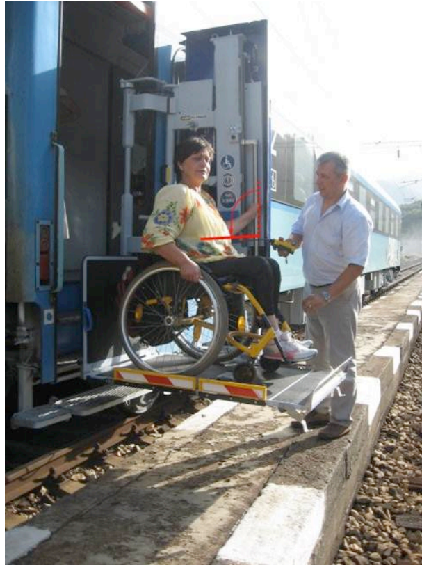
fig. 29 Additional foldable safety bar in order to increase the safety-feeling for WOs
