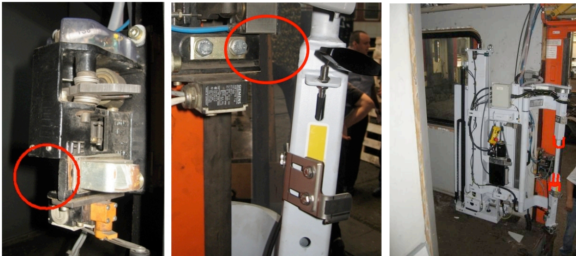
fig. 10 contact of slewing column with door-lock
