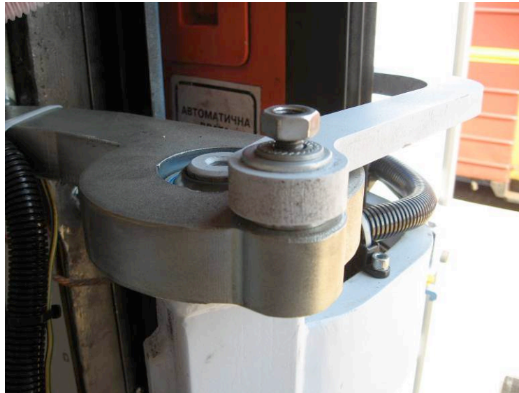
fig. 19 Loose Screws (swivelling mechanism)
