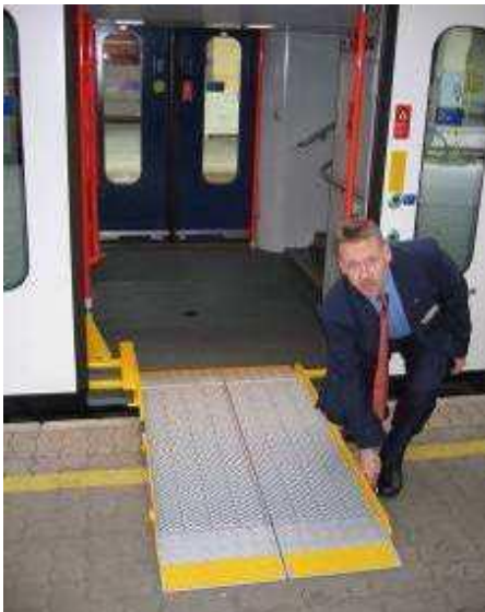
Picture 1 – Vehicle based ramp, ÖBB
