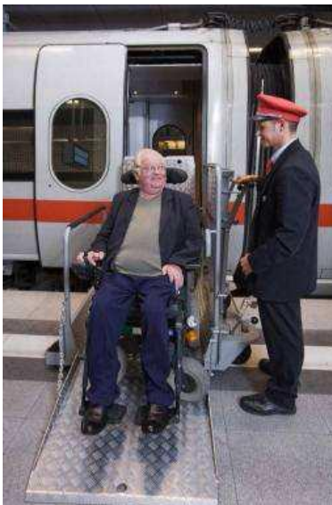
Picture 4 – Platform based lift, DB
