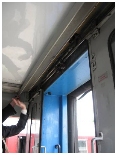
Figure 3.14: Space over the end door for door mechanism
