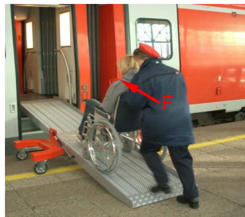
Figure 2.26: Required push (brake) force increases with the ramp slope
