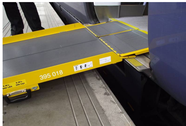
Figure 2.33 Ramp with raised edges in contrast colours – Southeastern Rail, UK
