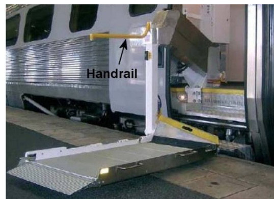
Figure 2.46: Handrail - Linear lift (Ratcliff Palfinger Trainlift RVT 300)
