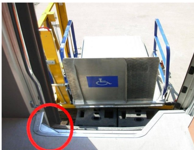
Figure 2.52 Permanent cover for dangerous stairs corner on the coach of Serbian Railways
