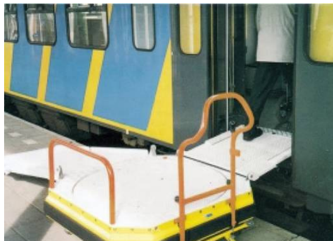
Figure 2.55: Collapsible side barrier- BraunAbility Millennium Series lift
