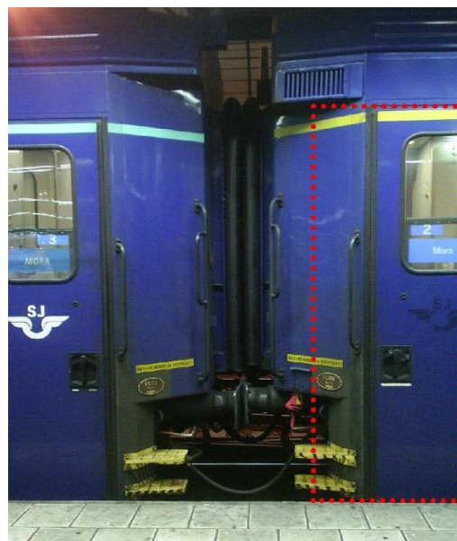
Figure 3.8: Position of the SJ doors compared to UIC coach doors
