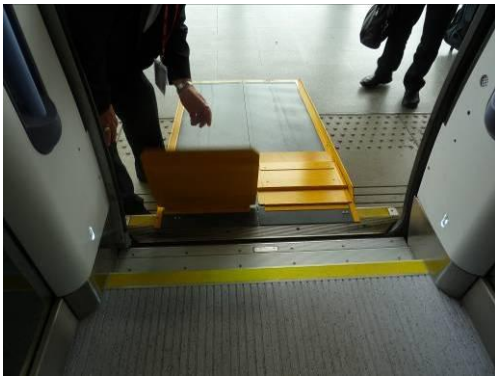
Pic. 20: Manual mobile Ramp (Port-a-Ramp, UK) to bridge the gap between the train and the platform (South Eastern Trains, England)
