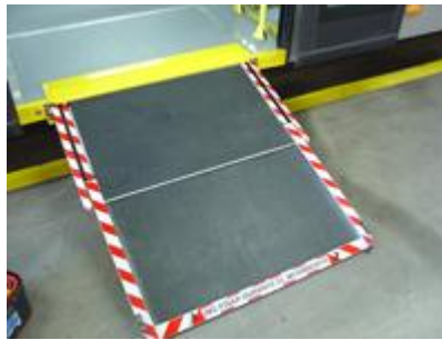
Pic. 33: Telescopic ramp, integrated into vehicle-floor (Masats)
