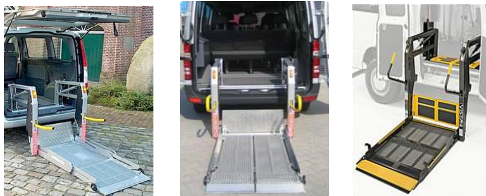
Pic. 99: Linear Lift, horizontal/vertical split-platform (left: AMF-Bruns, right: BraunCorp, )
